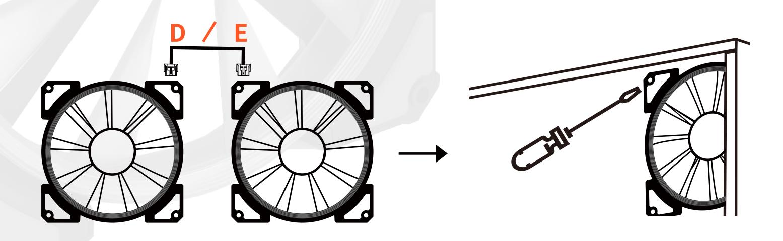
3. Use Addressable RGB Y-Cable to connect the fan and the motherboard. Please use RGB 3-Pin connector to an ADD RGB header, and 4-pin fan connector to a fan header on the motherboard. (Note: After connecting the Y-Cable with the motherboard, all the fan functions will be controlled by the motherboard. When connecting more than 5 fans, please use another Addressable RGB Y-Cable to connect the 6 or more fans.)
